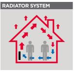
Convection causes drafts and uneven heat
